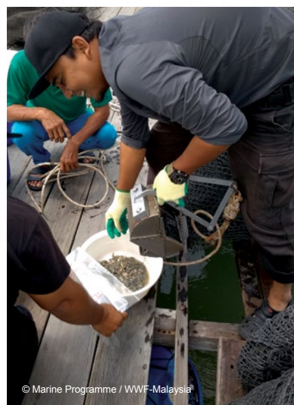
A grapple tool used to scoop the ocean floor for biodiversity and chemical analysis.
